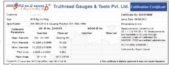
Calibration certificate issued with each gauge free of cost. It covers all important parameters of Threads. (Size: 21x10cms.)
